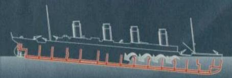
As each compartment filled, the bow sank deeper, and water flowed over the top of the bulkheads. With five compartments flooded, the ship could not survive
