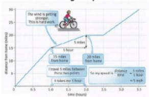
Calculate the gradient of the line on a distance-time graph to give you the speed of an object.
