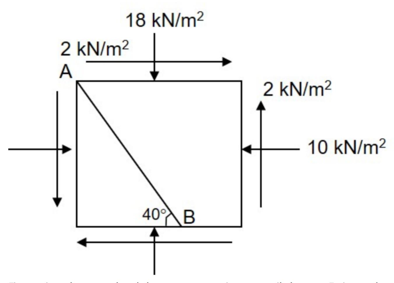
Figure gives the normal and shear stresses acting on a soil element. Estimate the normal stress (in kN/m²) acting on the plane AB.
