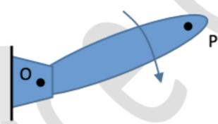
Determine the magnitude of the velocity of the point P if the distance from the pin O to P is 1.5 m.
