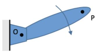
Determine the magnitude of the acceleration of the point P if the angular acceleration of the object is 4.5 rad/s² and the distance from the pin O to P is 1.5 m.
