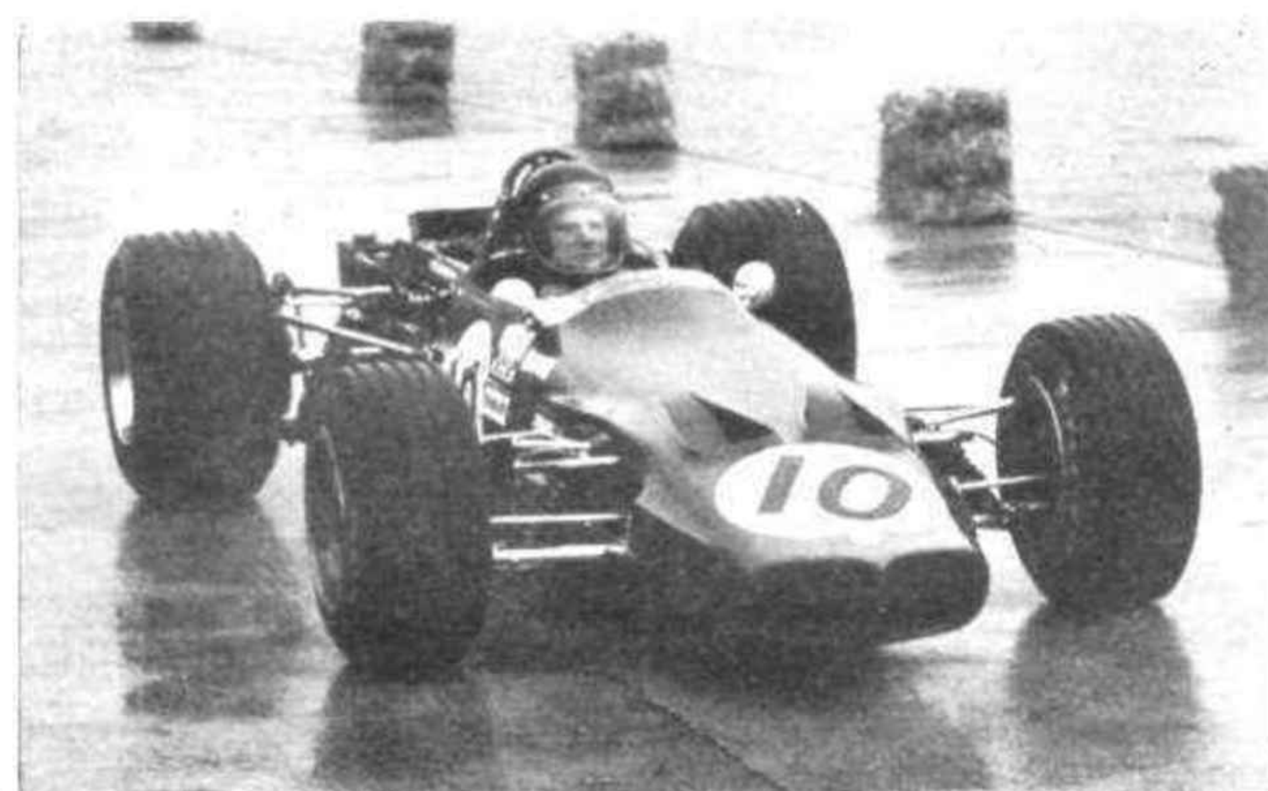
Brabham BT30 (left) and Lotus 59B (right) represent two different lines of thought in body design. Brabham drivers claim that the clean lines give the car extra top speed, but the Lotus is winning races without so much as a rear engine cover.
